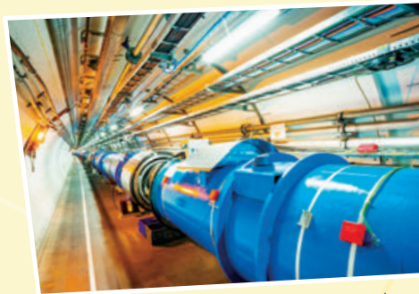
The Large Hadron Collider is a 16.6-mile-long circular tunnel. Powerful magnets inside it crash particles, like protons, at close to the speed of light.
